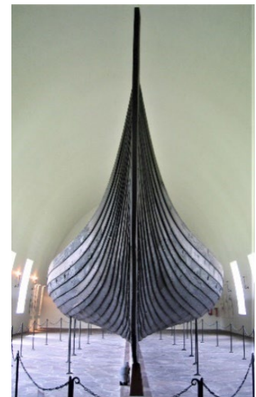
Gokstad longship showing clinker planking
